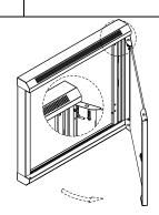
【2】Open the front door by key, pull the door latch downward, refer to the picture, remove the front door from front frame, put them separate for the preparation of the frame assembly.
