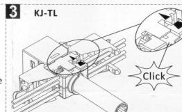
Insert the wires through the cap and seat the wires in the correct slots according to T568A or T568B. Match with the black triangle and align the cap with IDC until it clicked as shown.
