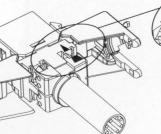
Match with the black triangle and align the cap with IDC until it clicked as shown. Press the cap down to IDC.
