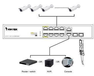
Use SFP, LC type transceiver with 100Mbps or 1Gbps transfer speed in Single mode (10km,30km,50km,80km) or Multi mode (0.5m or 2km) or Bidi (10km,30km,50km,80km).
