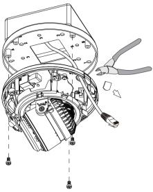
4-2-2. Connect the cables and install the top cover.
