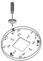
4-3-2. Install the camera to the mounting cap by turning it counter-clockwise so that the screw heads fit in the keyhole slots. Fasten the screws, and then connect the cables.
