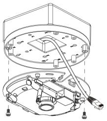
4-1-2. Connect the cables and install the top cover.
