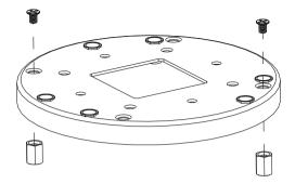
3. Install the mount cap to the junction box. Use screw holes specified on page 3 depending on the type of junction box.
