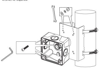
If you are installing a bullet camera directly to the bracket, use the M6 screws in the center. A hex crescent wrench is required.
