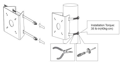
The 4 screw holes in the center are used for directly mounting the IB series bullet cameras.
