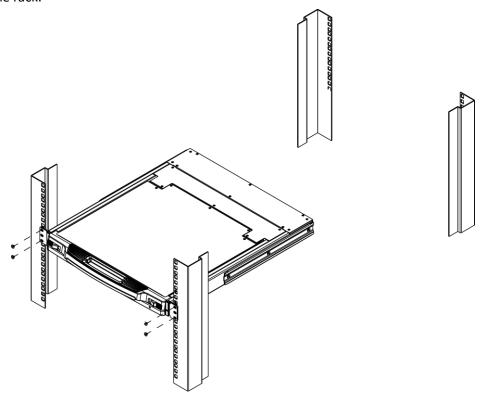
2. While the first person still holds the unit in place, the second person slides the left and right L-shaped brackets into the unit's side mounting brackets from the rear, installing four screws in the tabs to secure them in place.
