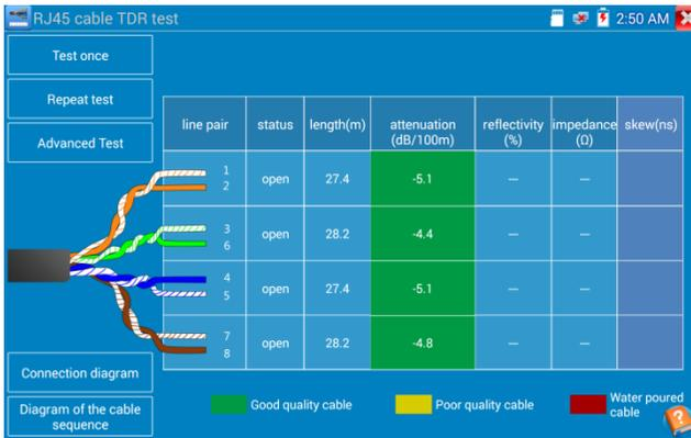
**Advanced Test:** Under RJ45 cable TDR test, it is able to test cable pair status, length, attenuation, reflectivity, impedance, skew and other parameters.
