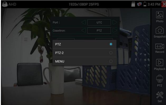
If to coaxial PTZ control the AHD camera, no parameters setting is needed.
