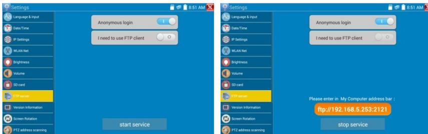
Start the FTP server and then input the tester's FTP address in the PC's address bar. This will enable the PC to read, copy and edit the files from the SD card without the use of SD card reader.
