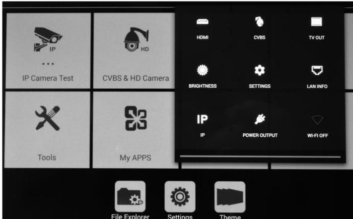
**HDMI:** Click HDMI to enter HDMI IN mode, it can convert test from analog to digital with dual test window IP & HDMI IN or Analog & HDMI IN.
