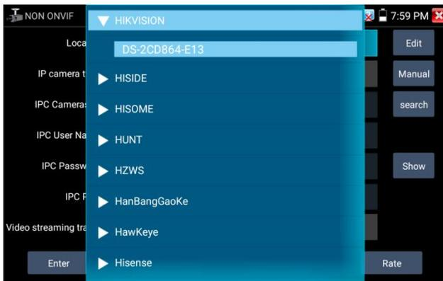
**Stream code:** When test camera via RTSP, you can select mainstream or sub stream to test (if camera’s RTSP have not been start or without, it will tip). If auto match fail, please switch to manually selecting.
