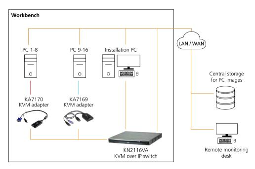
— DisplayPort Cable — Cat5 Cable — VGA Cable
